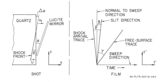
Fig. 2.5.--Definition of Parameters Used in Adjusting Streak Camera Data.
